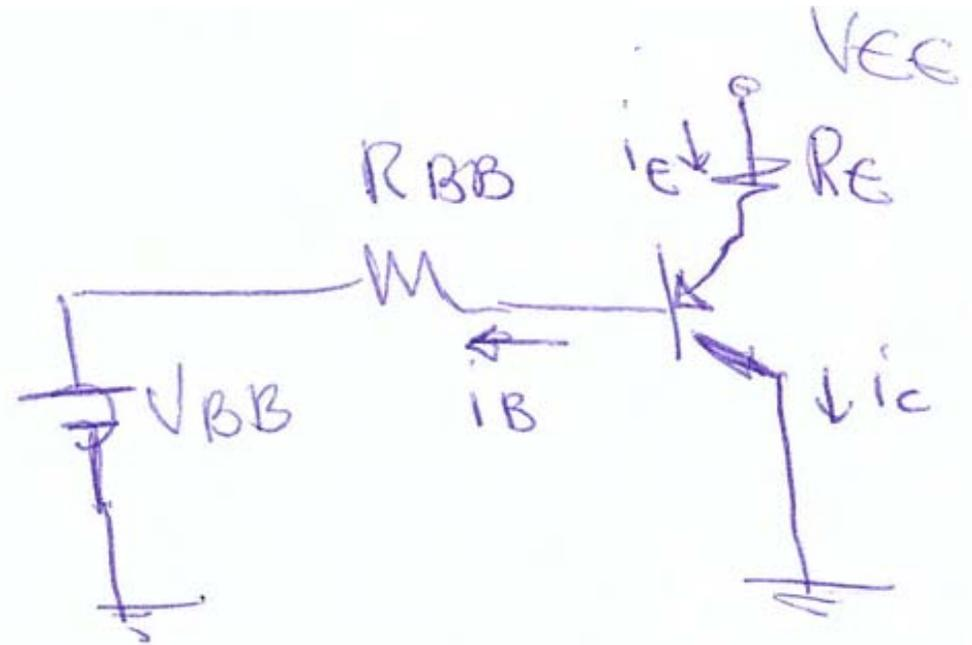
$$V_{EE} = R_E i_E + R_{BB} i_B + V_{EB} + V_{BB}$$
