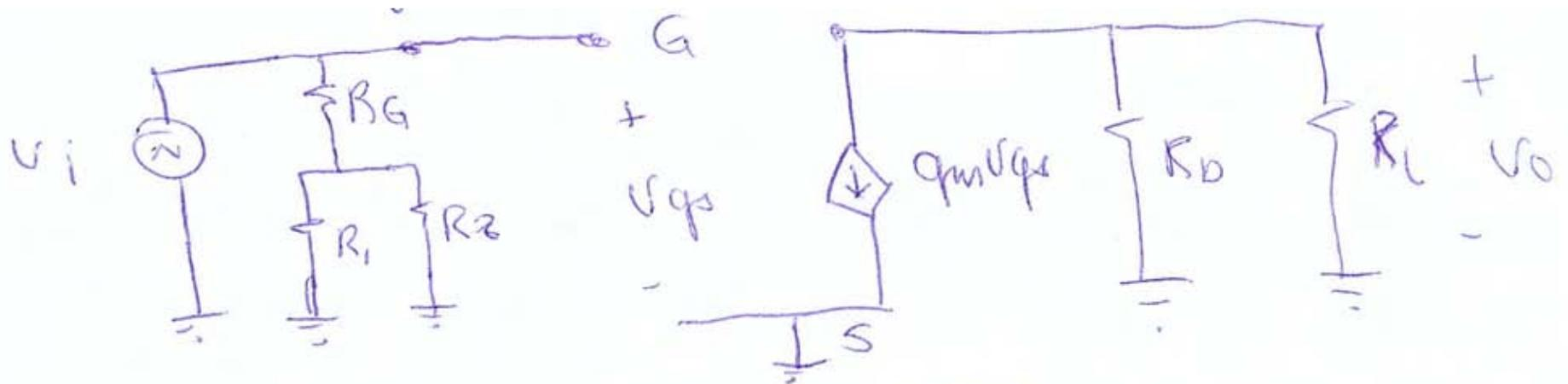
$$g_m = 2\sqrt{K I_D} = 2\sqrt{5 \times 1} = 4,47 \frac{\text{mA}}{\text{V}}$$
