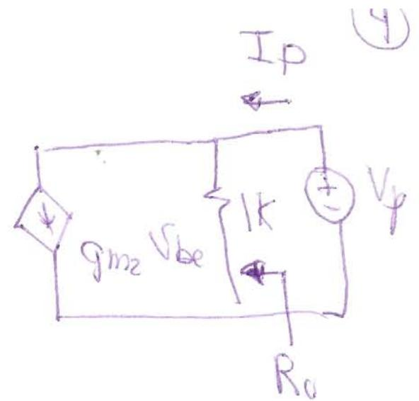
$$I_p = \frac{V_p}{R_o} + g_{m2} V_{be}$$
