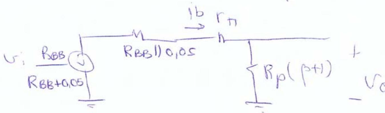
$$i_b = \frac{v_i R_{BB}}{(R_{BB} \parallel 0,05) + r_{\pi} + R_p(\beta+1)}$$
