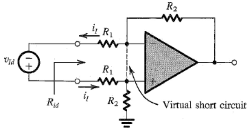
$$v_{id} = R_1 i_1 + v_{in} + R_1 i_1$$
