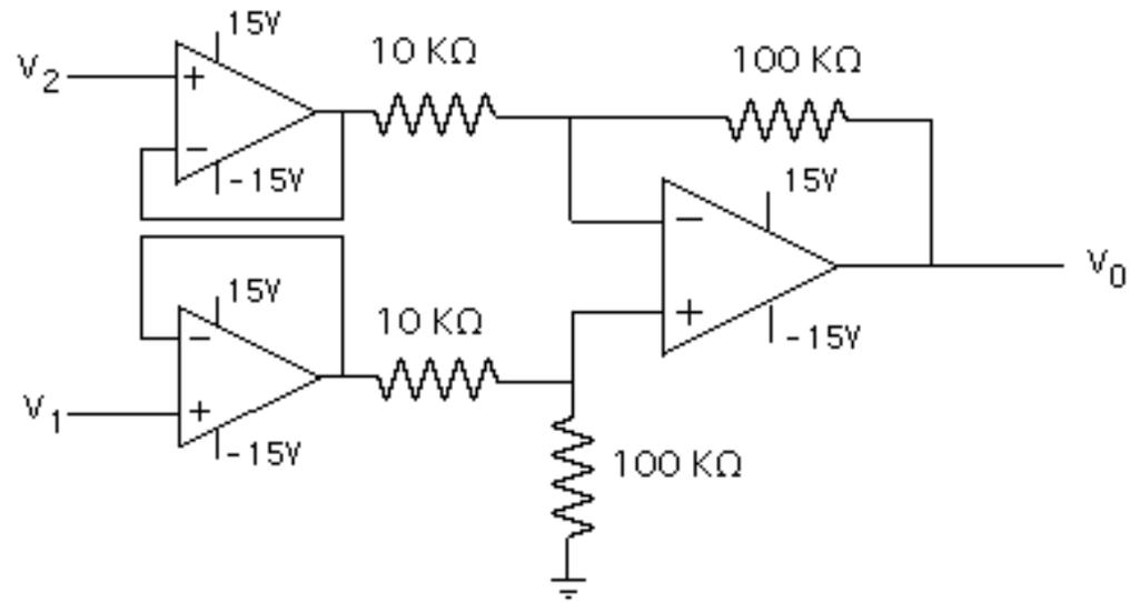
$$v_o = \frac{R_2}{R_1} (v_2 - v_1) = \frac{R_2}{R_1} E_0 = \frac{R_2}{R_1} \frac{V \Delta R}{40}$$
