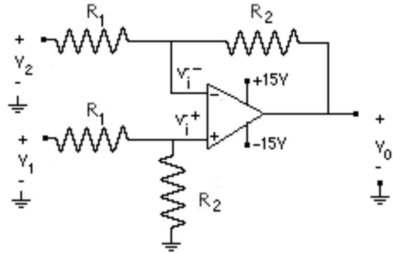
$$v_i = \frac{R_2}{R_1 + R_2} V_1$$
